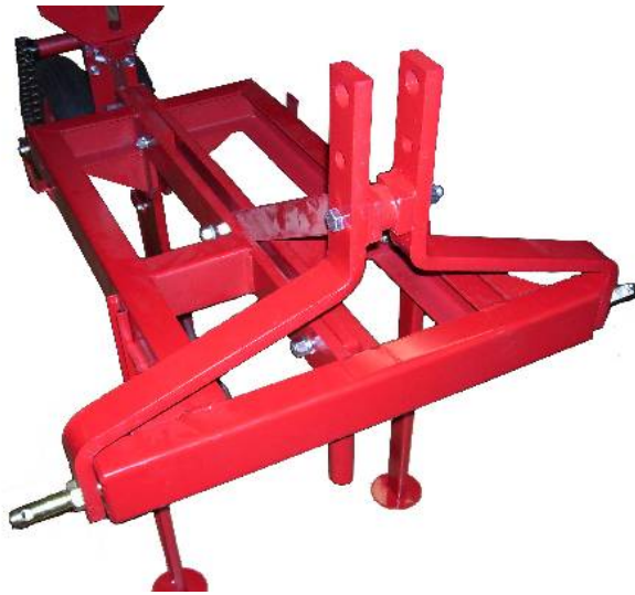
Illustration 4: Lift Arm Tripod as Installed
