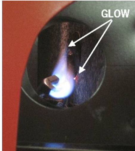
Illustration 4: Pilot Light Has Warmed Pad – Heater with Hard to See Heated Areas in Bright Light
