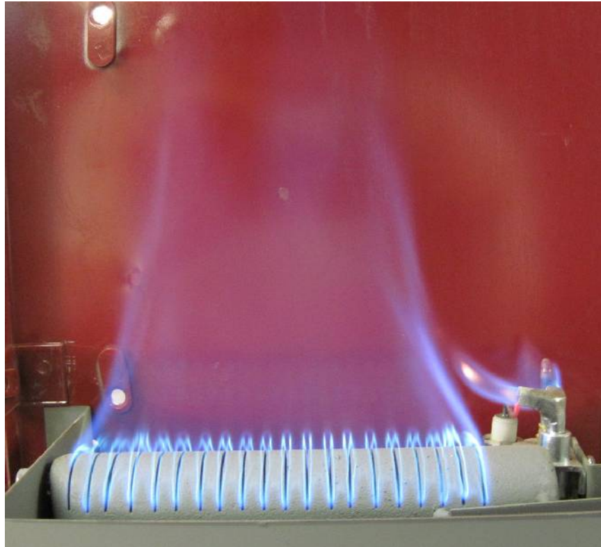
Illustration 3: Correctly Adjusted Burner Flame
